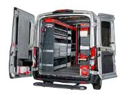
The grid dimensions allow all ORSY® elements to be combined with each other, including the vehicle interior equipment.
